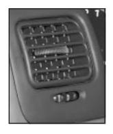
Use the air outlets located in the center and outboard sides of the instrument panel, to change the direction and amount of the air flowing through the vents.
